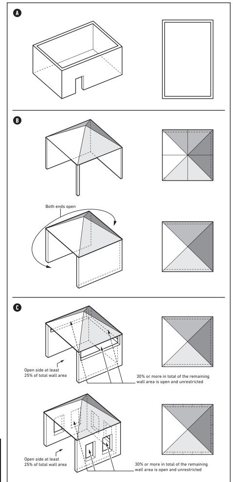
▲ IMPORTANT: This appliance shall only be used in an above ground open-air situation with natural ventilation, without stagnant areas, where gas leakage and products of combustion are rapidly dispersed by wind and natural convection.
