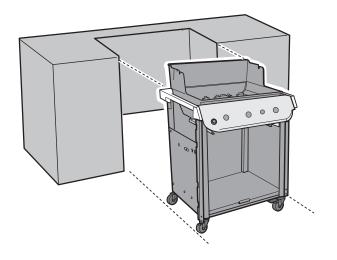
Push barbecue into cutout opening and lock the front casters. Rotate the front casters to tuck them beneath the cabinet.
