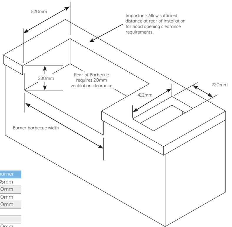
For built-in installations: islands, masonry, other non-combustible material structures.
