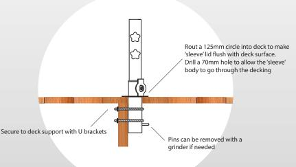
All hole sizes are indicative and should be adjusted depending on soil type. Final responsibility rests with the customer/installer.
